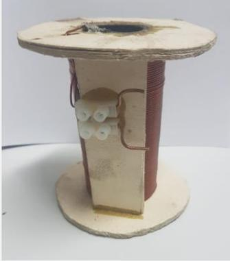
A photograph of a hand-wound inductor. It consists of a central PVC tube with a cardboard sleeve around it. The tube is wound with approximately 600 turns of thin copper wire. The assembly is mounted on a circular wooden base. Two wires extend from the bottom of the coil. |
